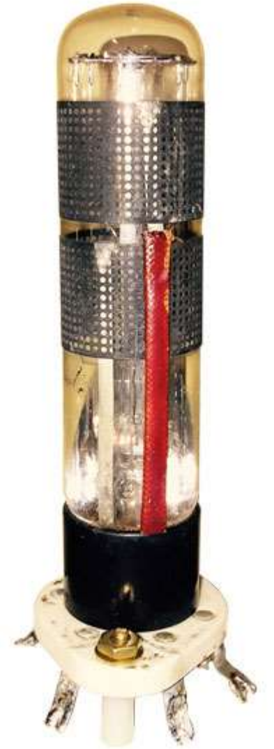
Collins/Amperex C100A “External Grid” tube
