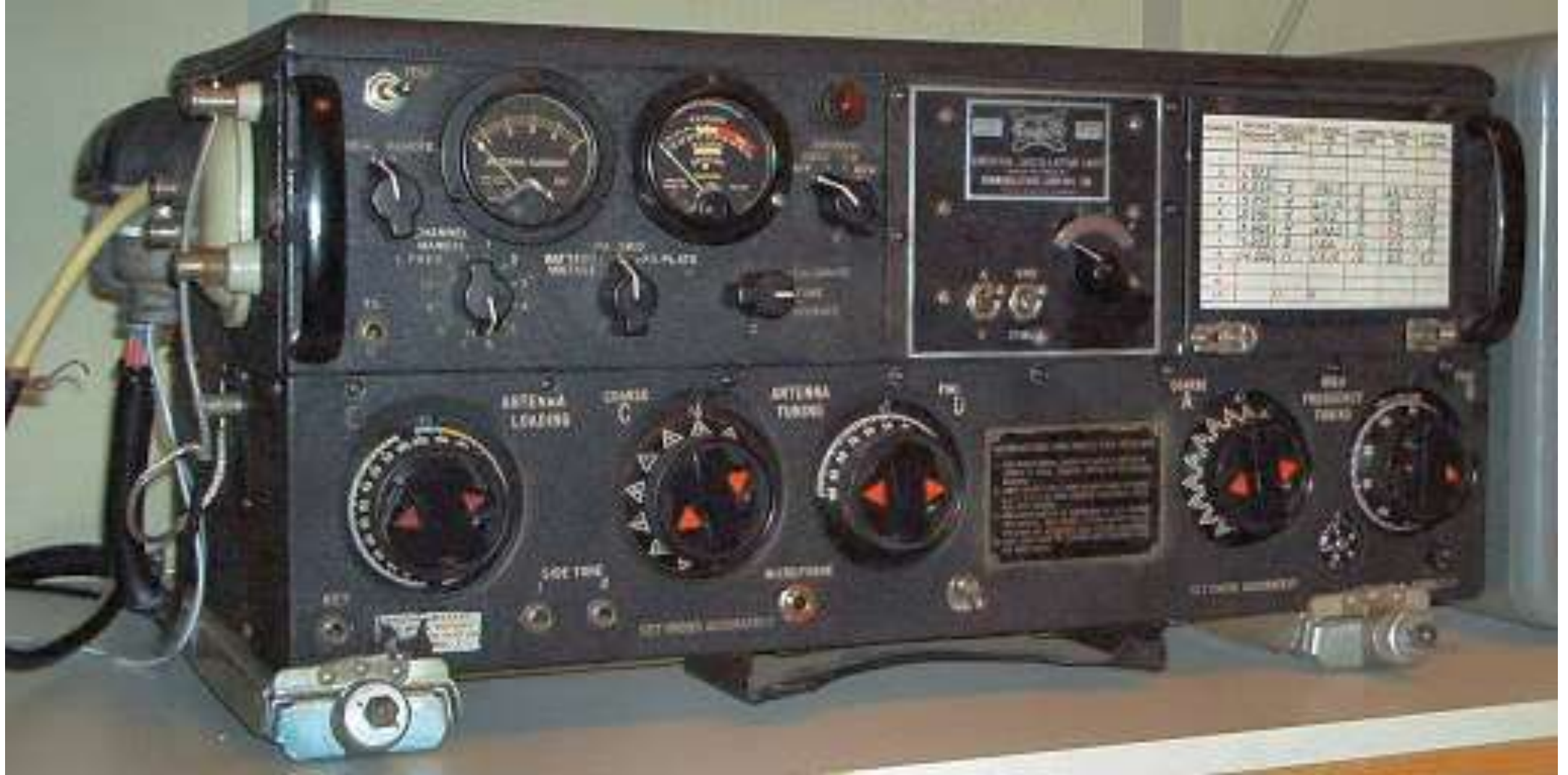
1941-1946 vintage AN/ART-13 Transmitter Up to 100W up to 18MHz 813 final. Was used into the 1970's First use of permeability tuning
