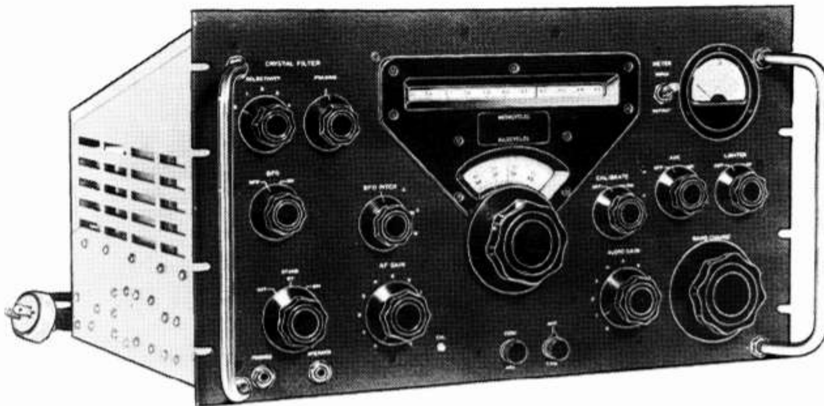
Collins 51J-4 receiver circa mid 1952-1954: 22 miniature tubes, dual conversion, mechanical filter, general coverage
