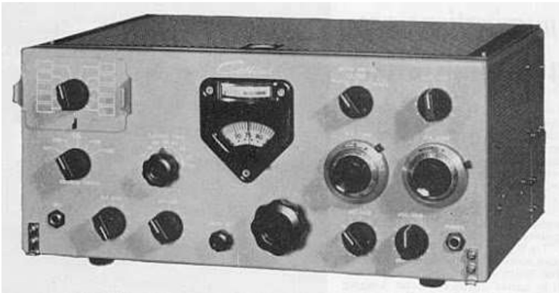
KWM-1 Transceiver 1957-76 14-30MHz, miniatures + 6146 final SSB, Mech filters.
