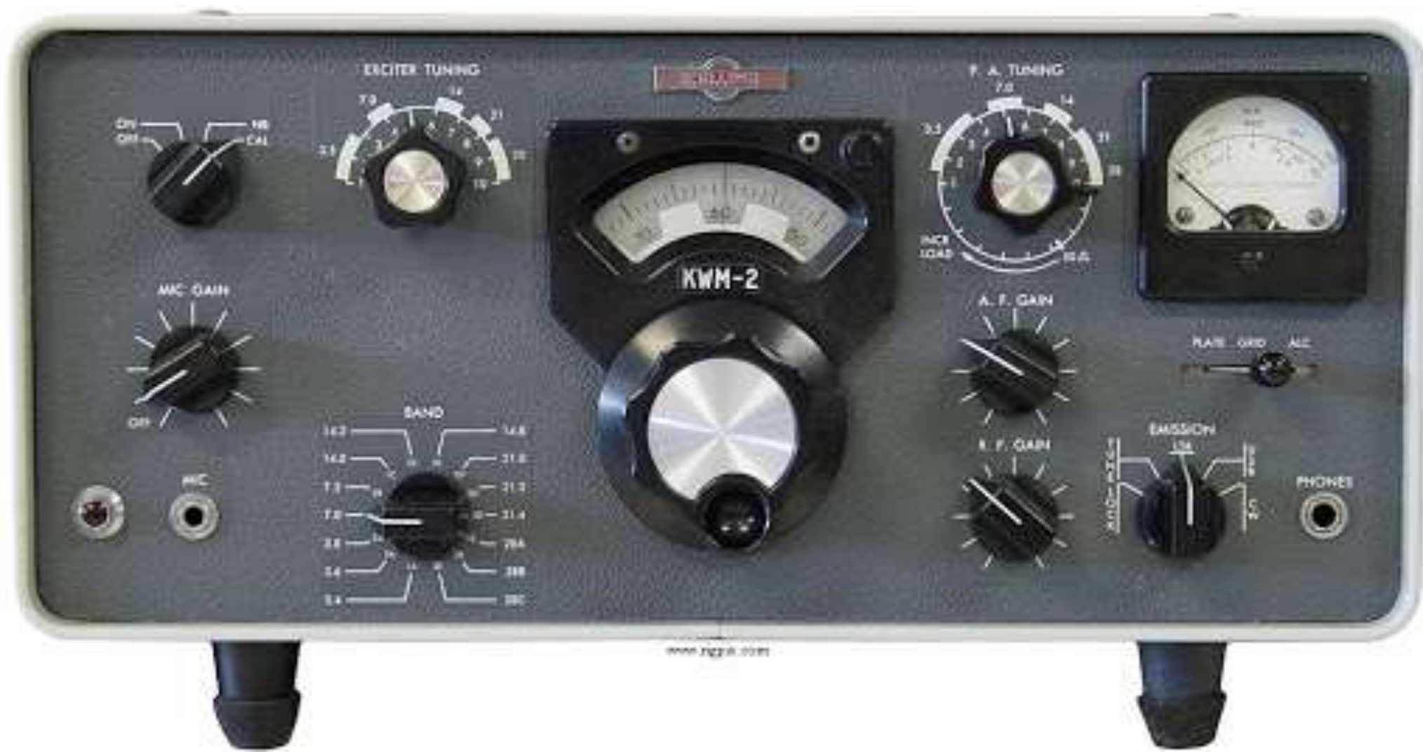
KWM2 Transceiver 17 tubes
