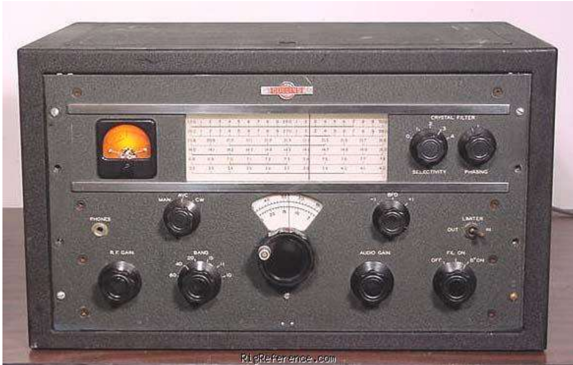
Collins 75A-1 receiver circa late 1947-49: 14 metal (octal) tubes, dual conversion, ham bands. "Their first modern receiver"
